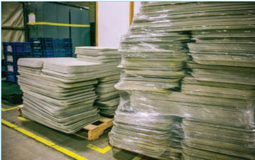
The material shown is what’s cut out of a RAV4 roof to make room for a sunroof. This “offcut” was once sent to a landfill for disposal, but now, it’s sent to PakFab, who turns it into returnable packaging bins. Called R3 Board, it performs better than the material it replaces.
