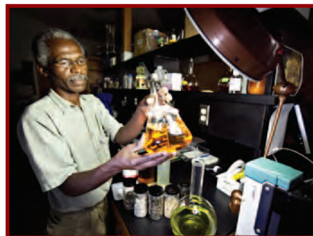
Dr. Ernst Cebert of Alabama A&M University's Department of Natural Resources and Environmental Sciences conducts a visual test on biodiesel to check for clarity. Toyota is a partner with the university in its biodiesel research project.
