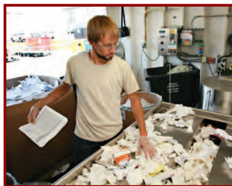
Employees at our plant in Princeton, Indiana, use a pulper to shred paper dishes from the cafeteria, paper break room waste, and bathroom paper towels and mix them with water to form a paper slurry. The pulp is sold to a paper recycling facility for use in products like paperboard and cardboard boxes.
