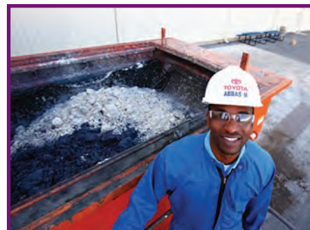
Using a gravity filter to dewater paint sludge reduces the amount of waste sent off-site for treatment, and allows for the remaining sludge to be used as a recyclable material.
