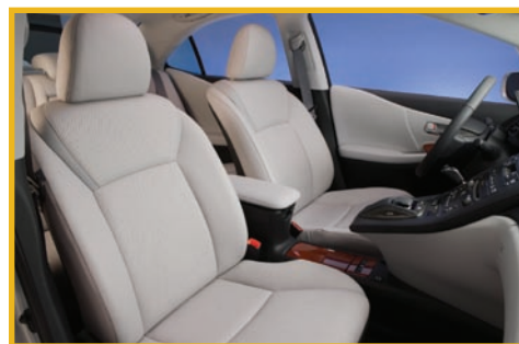
Ecological Plastics are used on interior parts in a number of our vehicles. Both the 2010 Prius and the new Lexus HS 250h have seat cushions that contain foam made of a material derived from castor oil.
