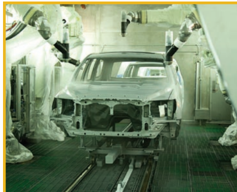
Conversion of the paint booths at our plant in Princeton, Indiana, to water-borne systems is expected to reduce VOC emissions by 27%.
