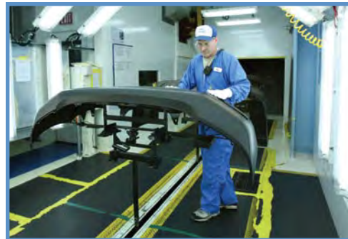
An employee at our plant in Indiana inspects a bumper that has just been painted with a water-based primer.
