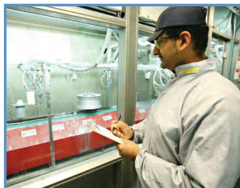
The paint booth at our plant in Delta, British Columbia, is equipped with electrostatic bell and high volume low pressure spray technologies, which increase transfer efficiency of the paint to the wheel and reduce waste paint and VOC emissions.
