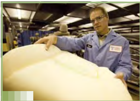
Toyota is using a renewable resource — soybeans — in the foam of passenger seats in the Toyota Corolla and the Lexus RX.
