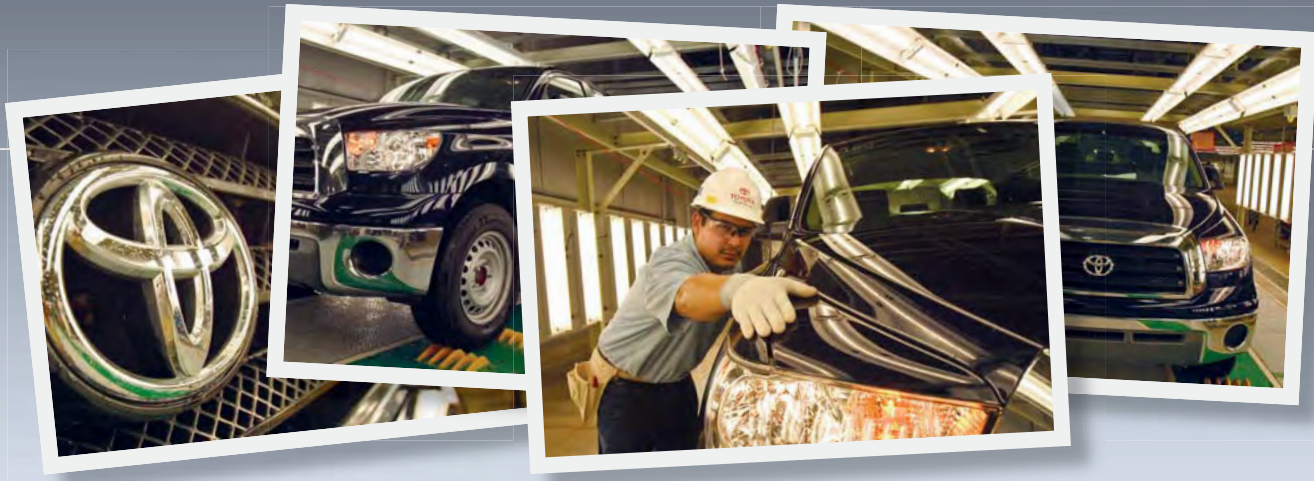
During startup trials at Toyota Motor Manufacturing, Texas, a team member checks a Tundra for leaks after it exits a shower test that uses recycled water.
