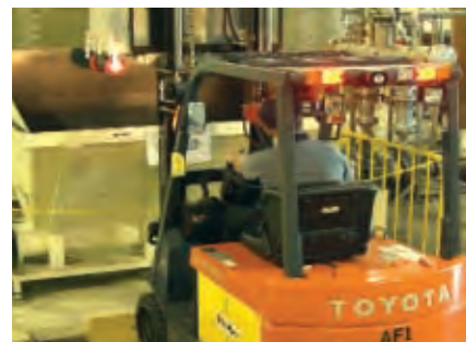
Team Member Ricky Dale places a cart full of metal sludge into the briquetter machine at Toyota Motor Manufacturing, Alabama, Inc., Hunstville, Alabama. The briquetter makes it easier to recycle sludge and prevents it from ending up in a landfill.
