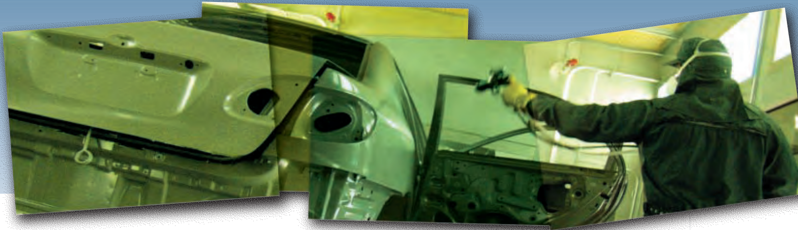
Team Member Ron Fratoni sprays inside of car doors in a paint booth at New United Motor Manufacturing, Inc., Fremont, California.
