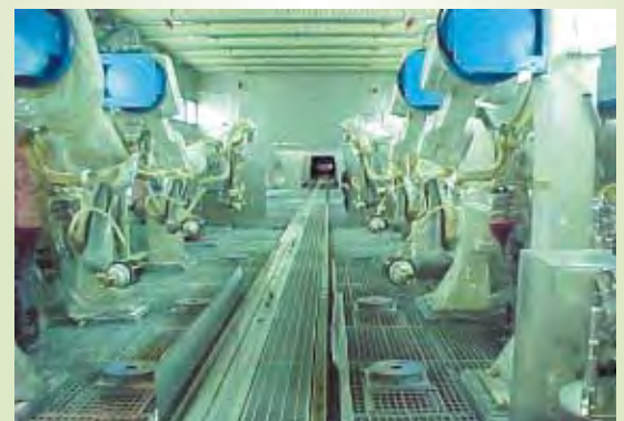
Toyota continues to reduce solvent emissions by installing the latest painting technology, such as this state-of-the-art paint booth.
